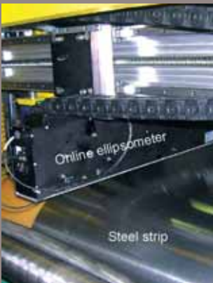
On line spectroscopic ellipsometer for real time thickness and composition measurement of nanometric film on a roll-to-roll line.
